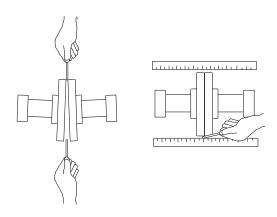
Figure B-4. Aligning Non-Spider-Type Couplings
