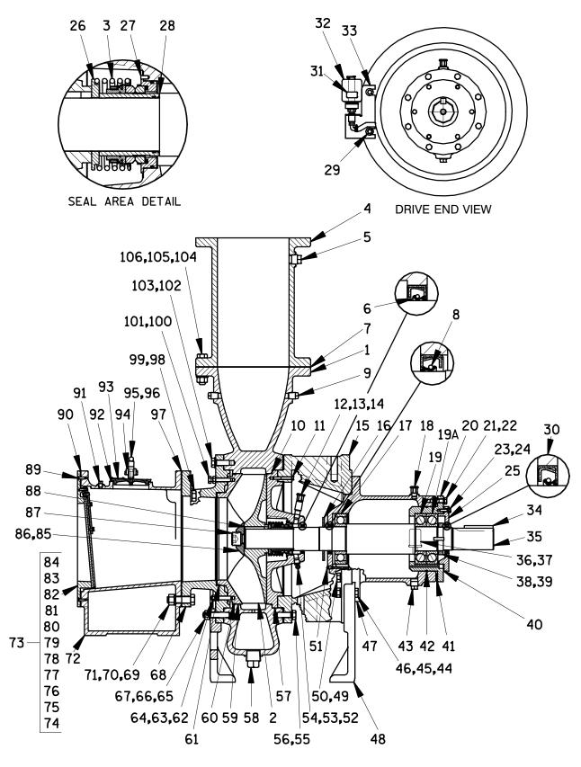
Figure E-1. Pump Model 112C60-B
