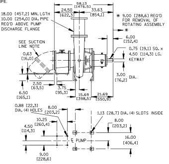
Figure B-1. Pump Model 112C60-B
