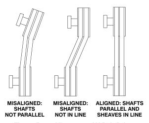
Figure B-5. Alignment of V-Belt Driven
