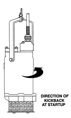
Figure 1. Checking Pump Rotation
