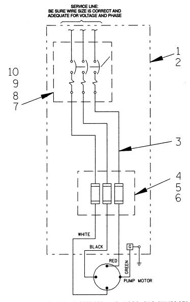
Figure 9. Pictorial Diagram - 47631-066 (460V 3P) and 47631-078 (575V 3P) Control Boxes
