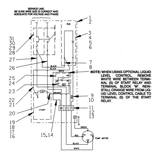
Figure 7. Pictorial Diagram - 47631-068 (115V 1P) And 47631-069 (230V 1P) Control Boxes INTERNAL PARTS LIST
