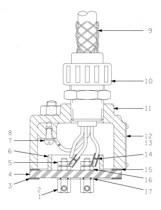
Figure 2. 47367-051 Terminal Housing And Cable Assembly
