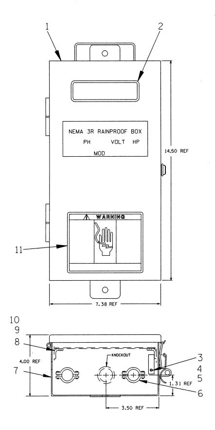
Figure 3. Control Box Dimensions
