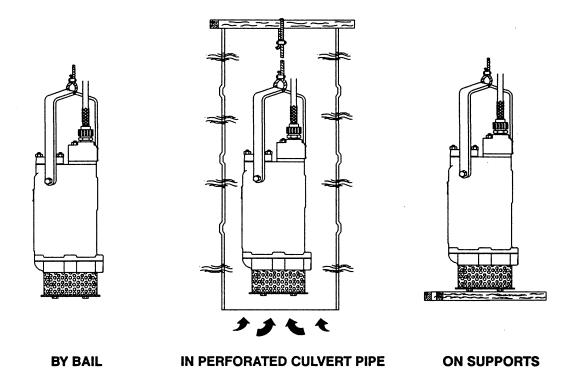
Figure 2. Typical Pump Installations
