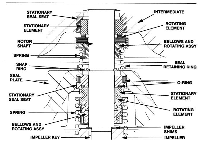
Figure 3. 46512-036 (Lower) And 25271-824 (Upper) Seal Assemblies
