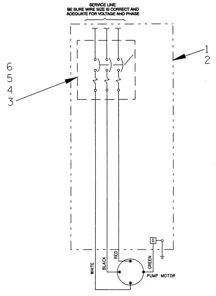
Figure 8. Pictorial Diagram - 47631-067 (230V 3P) Control Box
