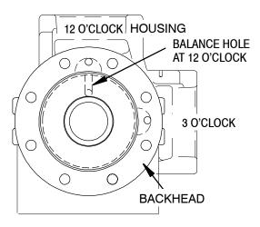
Figure E-5. Housing/Backhead Alignment
