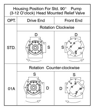
Figure B-1. Typical Port Positions & Rotation
