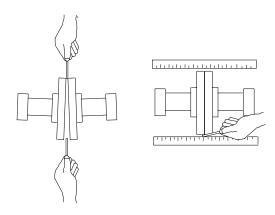
Figure B-3. Aligning Non-Spider Type Coupling
