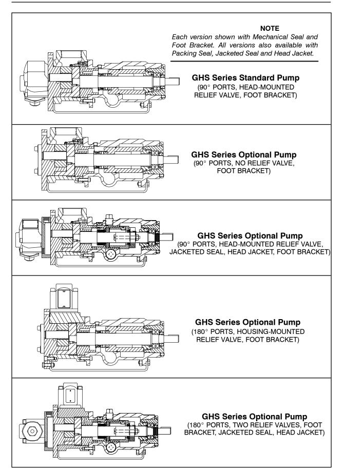
Figure E-2. Assembled GHS Pump Models
