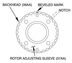
Figure E-6. End Clearance Adjustment
