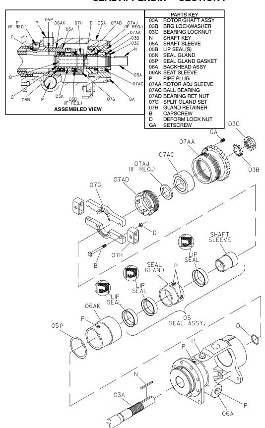
Figure F-10. Cartridge Lip Seal (Option 65E)
