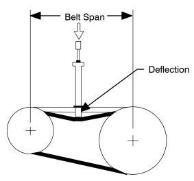
Figure B-5. Belt Tension Measurement
