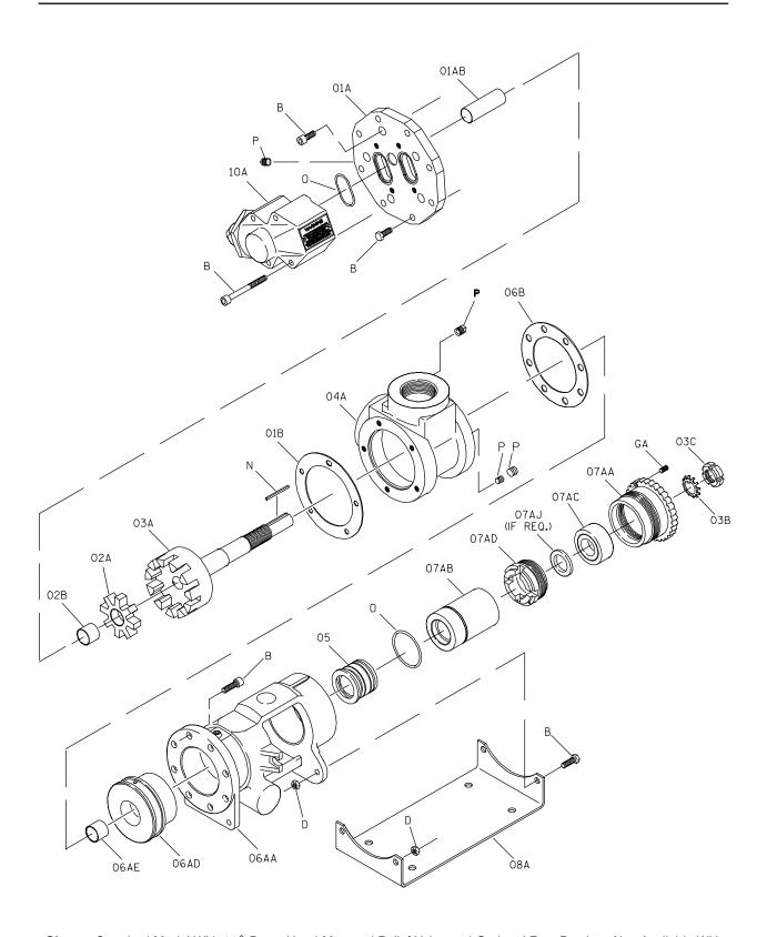
**Shown:** Standard Model With  $90^{\circ}$  Ports, Head-Mounted Relief Valve and Optional Foot Bracket. Also Available With  $180^{\circ}$  Ports And/Or Jacketed Seal, Head Jacket, Housing-Mounted Relief Valve. A Coverplate Kit Replaces Either Relief Valve When Not Used.
