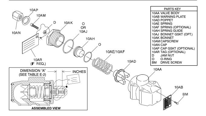
Figure E-7. Pressure Relief Valve Assembly
