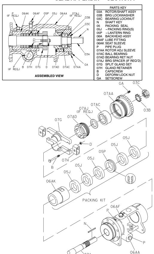
Figure F-11. Standard (And Optional 65Q) Packing Seals
