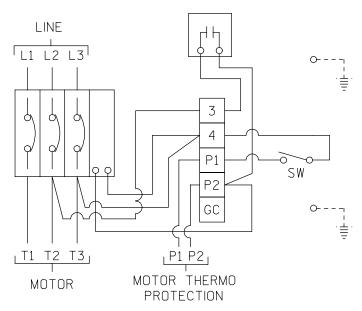
Figure B-5. Mounting Plate Wiring Schematic
