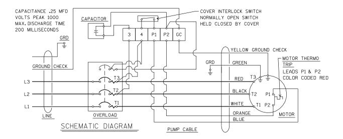
Figure B-3. Pump Power Cable Connection Diagram (All Models)
