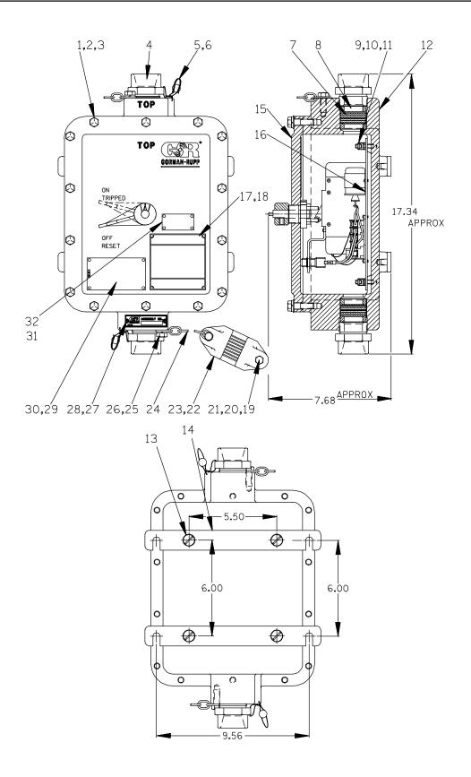
Figure B-1. NEMA Type 10 MSHA Certified Control Box Dimensions
