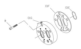
Figure E-2. Typical Head Jacket Assembly
