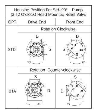
Figure B-1. Typical Port Positions & Rotation
