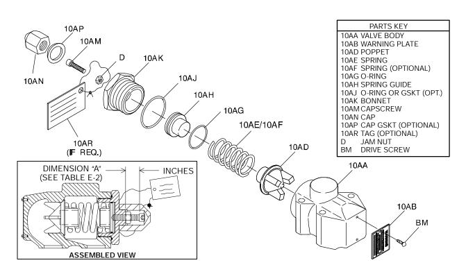
Figure E-6. Pressure Relief Valve Assembly
