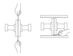
Figure B-3. Aligning Non-Spider Type Coupling
