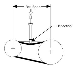
Figure B-5. Belt Tension Measurement
