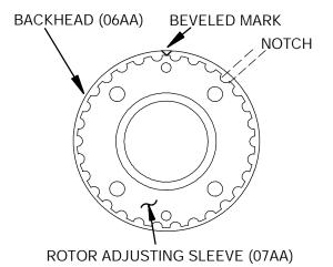
Figure E-5. End Clearance Adjustment
