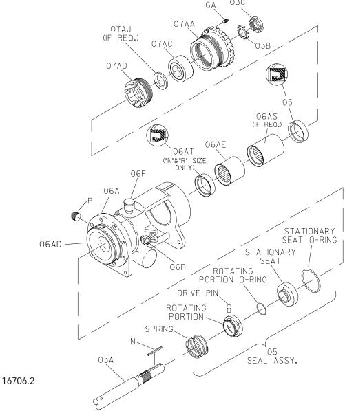
Figure F-2. Lug Drive (Option 62A And 62B) Mechanical Seals
