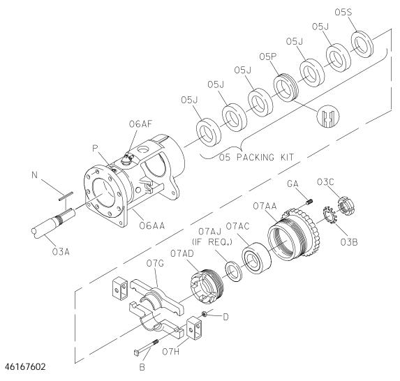
Figure F-4. Packing Seal (Option 65P)
