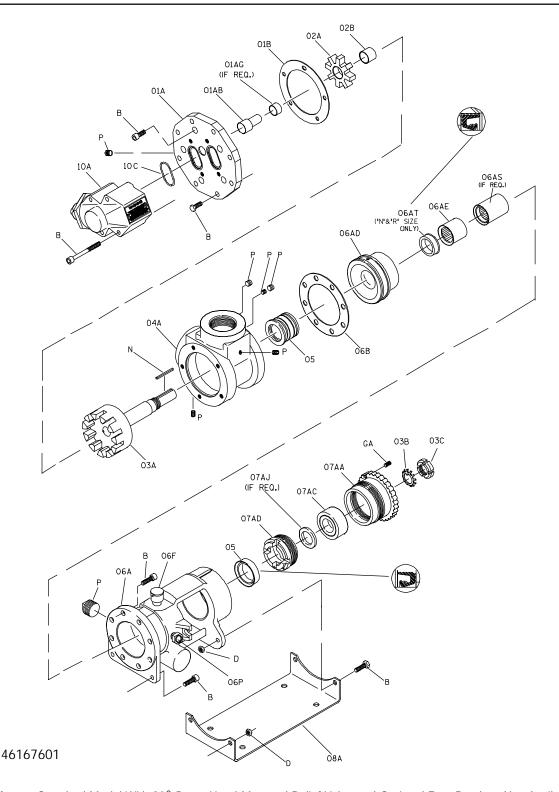
**Shown:** Standard Model With 90° Ports, Head-Mounted Relief Valve and Optional Foot Bracket. Also Available With 180° Ports And/Or Head Jacket, Housing-Mounted Relief Valve. A Coverplate Kit Replaces Either Relief Valve When Not Used.
