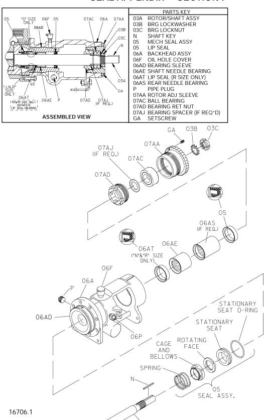
Figure F-1. Standard Type 43 Mechanical Seal
