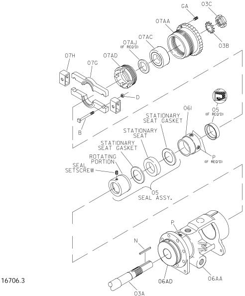
Figure F-3. Positive Locking/Clamped Seat Seal (Option 62C)
