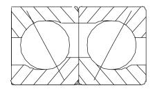
Figure E-2. Correct Bearing Mounting
