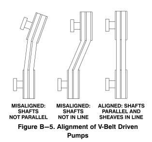
Tighten the belts in accordance with the belt manufacturer's instructions. If the belts are too loose, they will slip; if the belts are too tight, there will be excessive power loss and possible bearing failure. Select pulleys that will match the proper speed ratio; overspeeding the pump may damage both pump and power source.
