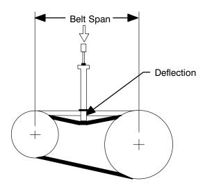
Figure B–6. Belt Tension Measurement
