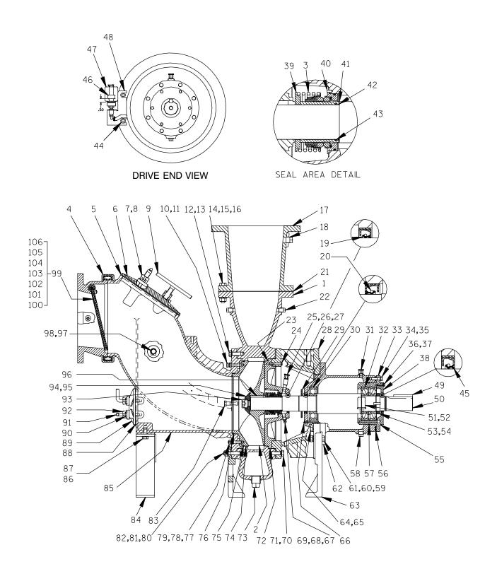
Figure E–1. Pump Model 112G60–B
