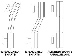
NOT PARALLEL NOT IN LINE SHEAVES IN LINE Figure 4C. Alignment of V-Belt Driven Pumps
