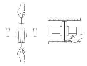
Figure 4B. Aligning Non-Spider Type Couplings
