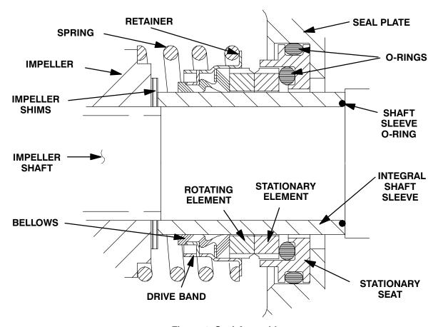
Figure 4. Seal Assembly
