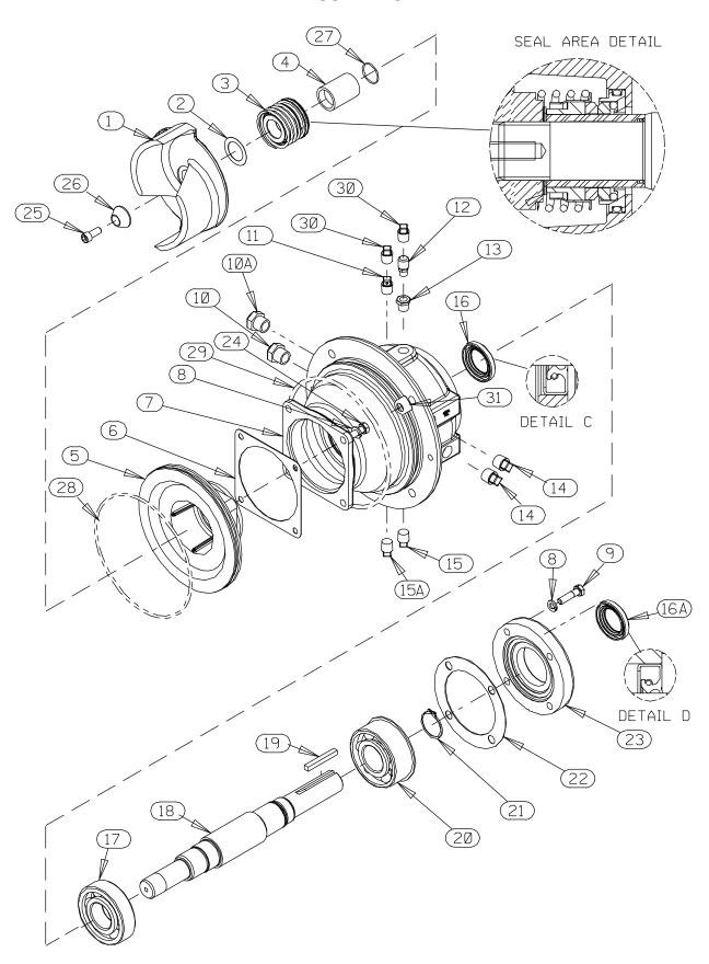
Figure 2. Repair Rotating Assembly
