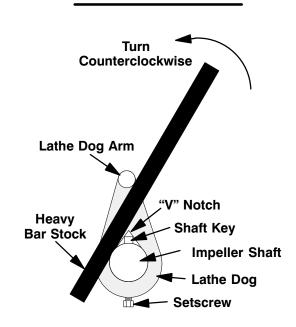
Figure 3. Loosening Impeller
