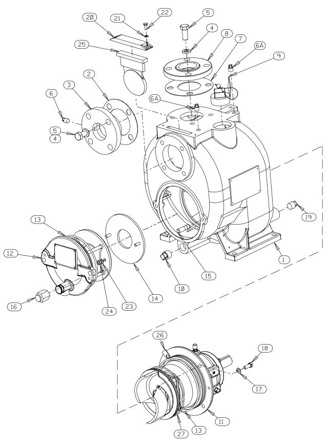
Figure 1. Pump Model T2A71-B, Including /F, /FM
