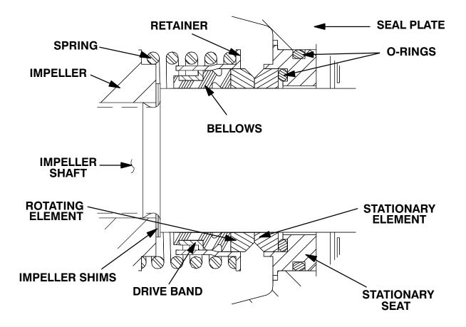
Figure 6. Seal Assembly
