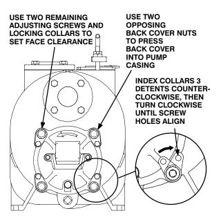
Figure 9. Installing and Adjusting Back Cover
