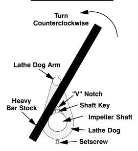
Figure 3. Loosening Impeller
