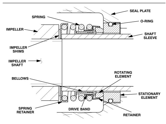
Figure 6. Seal Assembly
