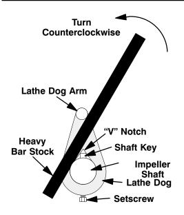
Figure 5. Loosening Impeller
