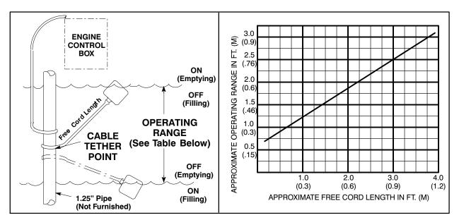
Figure 3. Float Switch Data
