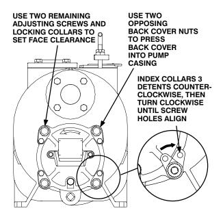
Figure 11. Installing and Adjusting Back Cover
