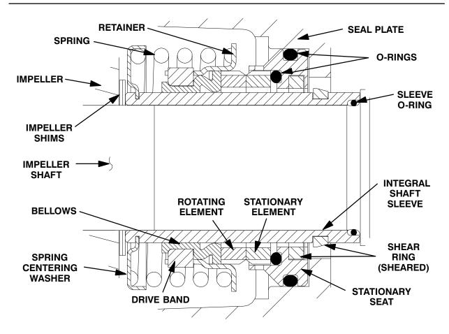
Figure 8. 46513–151 Cartridge Seal Assembly
