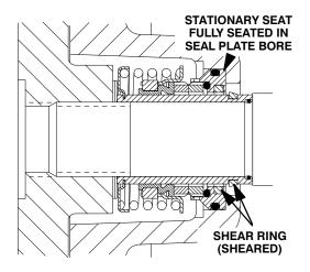
Figure 10. Seal Fully Installed
