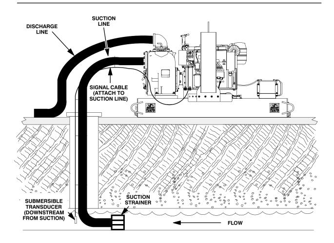
Figure 4. Typical Submersible Transducer Installation
