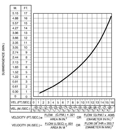
Figure 1. Recommended Minimum Suction Line Submergence vs. Velocity
