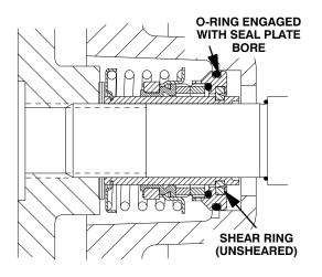
Figure 9. Seal Partially Installed
