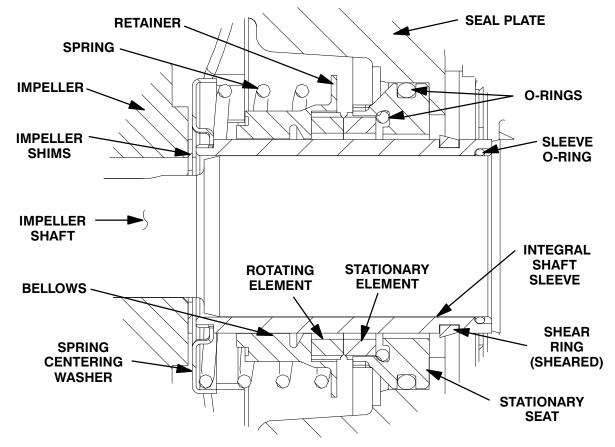
Figure 8. Cartridge Seal Assembly
