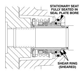
Figure 10. Seal Fully Installed
