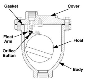
Figure 6. Priming Chamber
