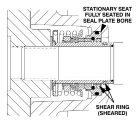
Figure 11. Seal Fully Installed
