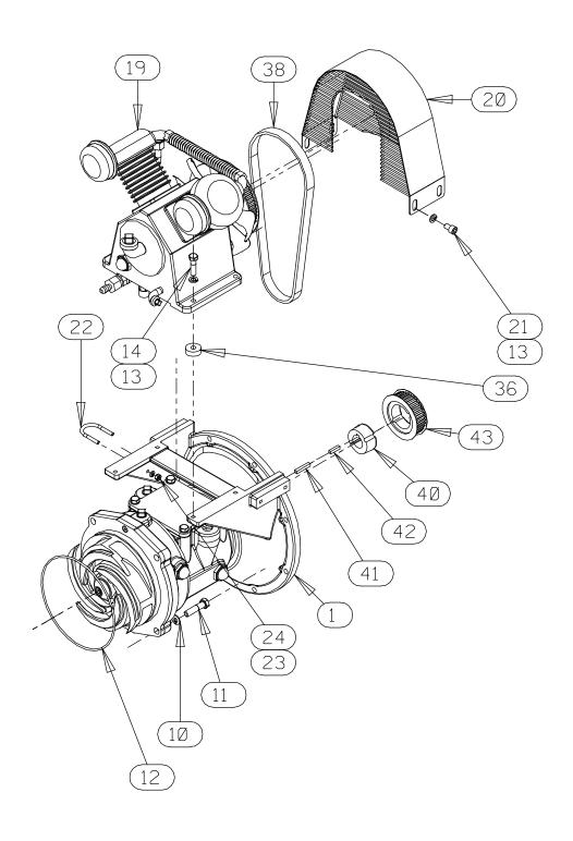
Figure 4. Pump End Assembly PAV3C60C-B-(E10) (Cont'd)
