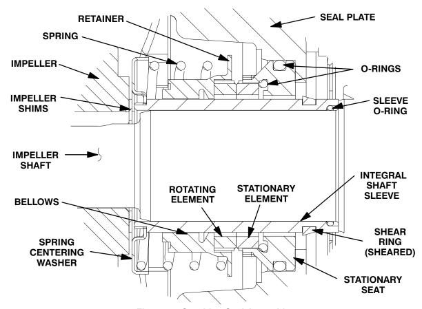
Figure 9. Cartridge Seal Assembly
