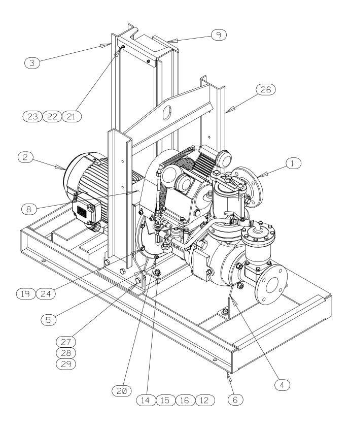
Figure 1. Pump Model PAV3C60C-B-E10 460/575/3
