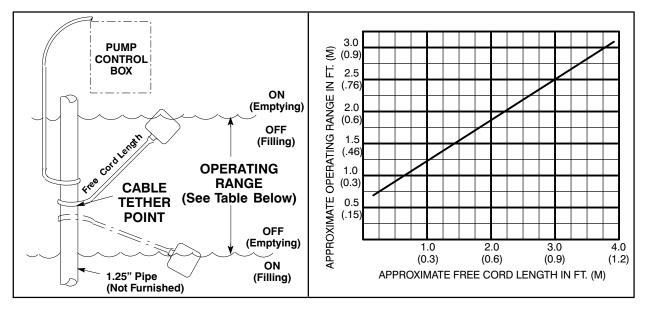
Figure 4. Float Switch Data
