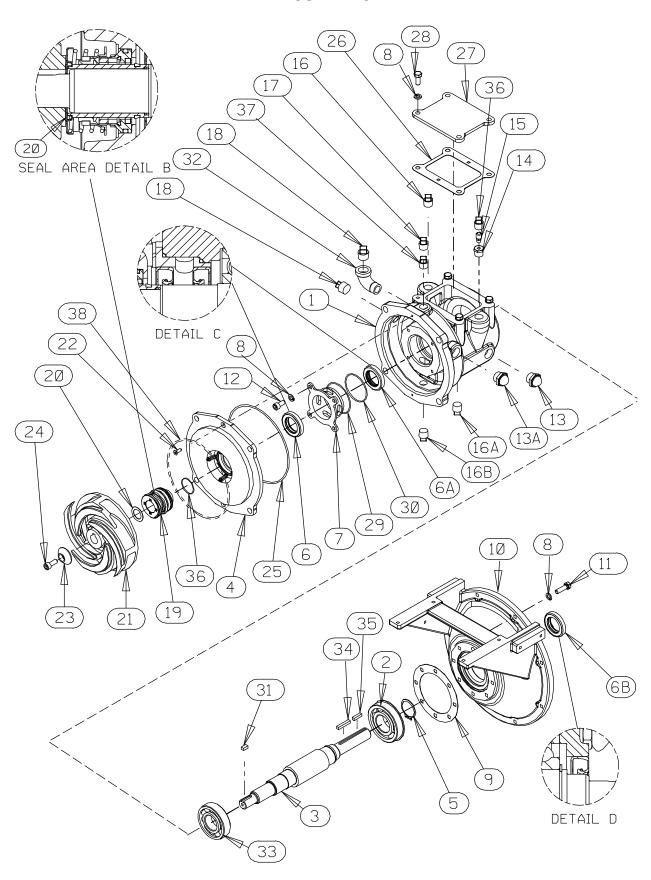
Figure 5. 44163-526 Repair Rotating Assembly
