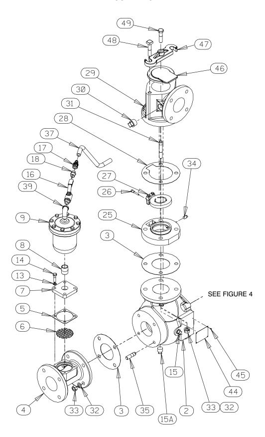
Figure 3. Pump End Assembly PAV3C60C-B-(E10)
