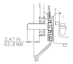
Figure 8. Drive Sprocket Positioning
