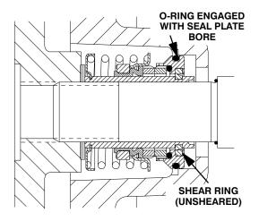
Figure 10. Seal Partially Installed
