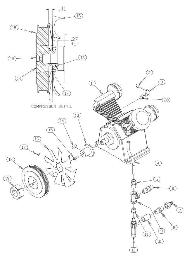
Figure 6. 46181-908 Air Compressor Assembly
