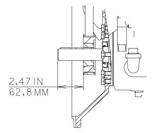
Figure 8. Drive Sprocket Positioning
