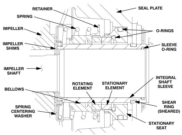
Figure 9. Cartridge Seal Assembly
