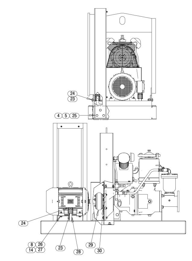
Figure 2. Pump Model PAV3C60C-B-E10 460/575/3 (Cont'd)
