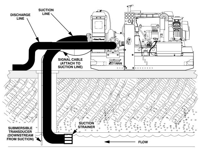
Figure 5. Typical Submersible Transducer AutoStart Pump Installation
