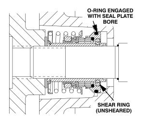
Figure 10. Seal Partially Installed
