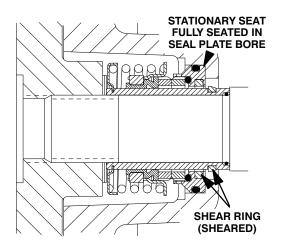
Figure 11. Seal Fully Installed
