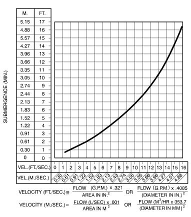
Figure 2. Recommended Minimum Suction Line Submergence vs. Velocity
