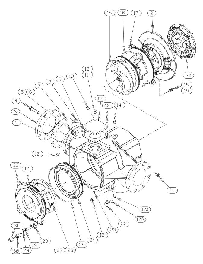
Figure 4. 66F60–(SAE 3/10) Pump End Assembly
