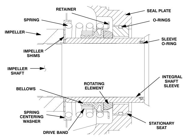
Figure 10. Seal Assembly
