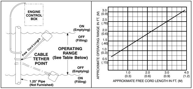
Figure 3. Float Switch Data
