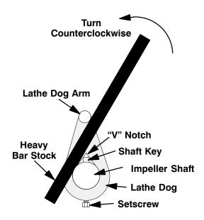
Figure 9. Loosening Impeller
