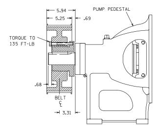
Figure 11. Bushing and Sprocket Installation
