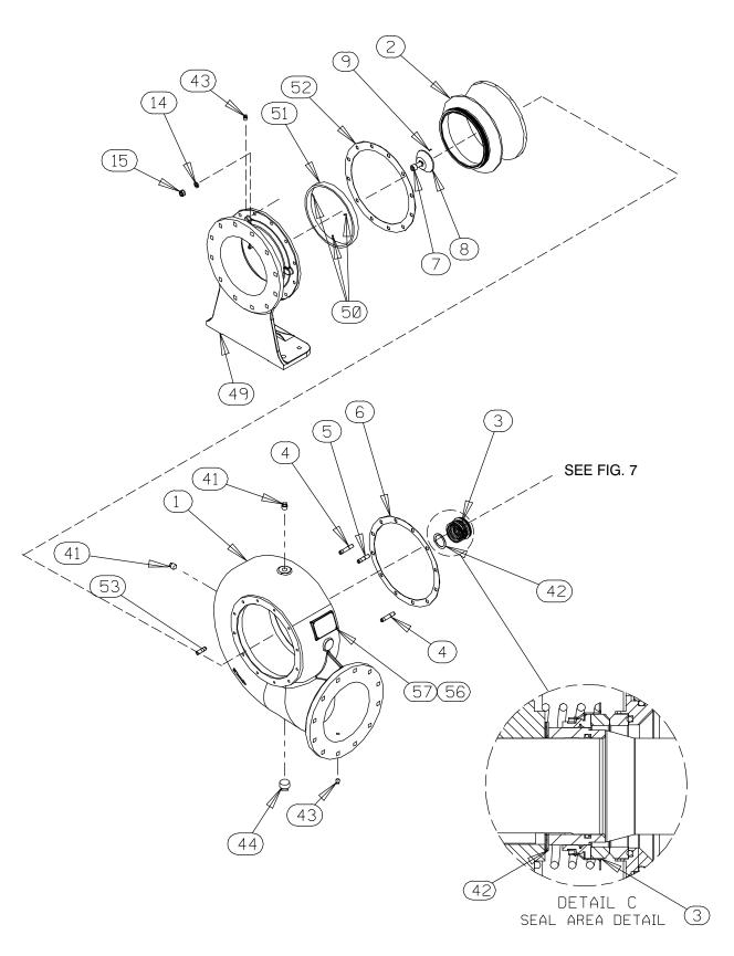
Figure 6. 612M60-B Pump Model Assembly
