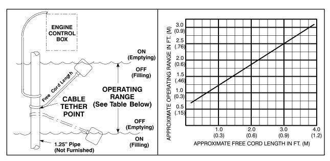
Figure 3. Float Switch Data
