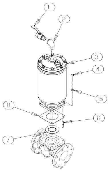
Figure 8. 48275-006 Priming Chamber Kit
