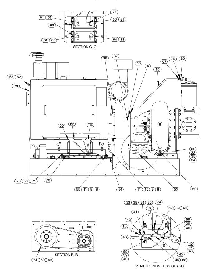
Figure 3. 46183-021 Pump Subassembly (Cont'd)
