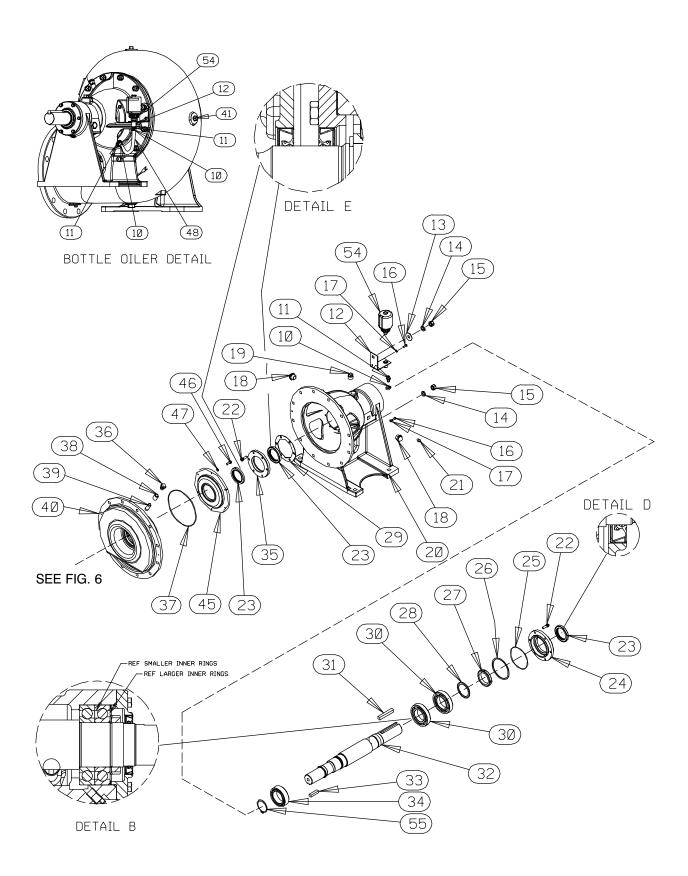
Figure 7. 612M60-B Pump Model Assembly (Cont'd)
