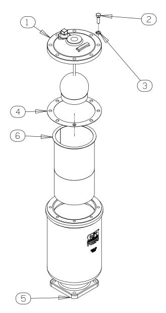
Figure 9. 46112—709 Priming Chamber Assembly PARTS LIST
