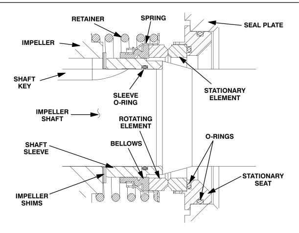
Figure 13. Seal Assembly
