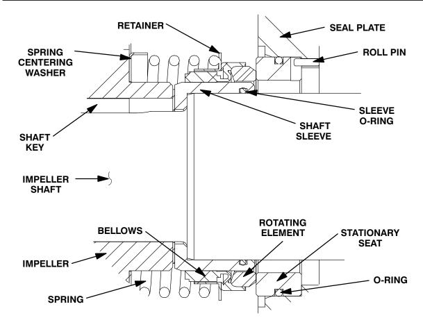
Figure 11. Seal Assembly
