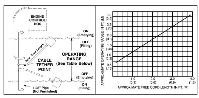
Figure 3. Float Switch Data
