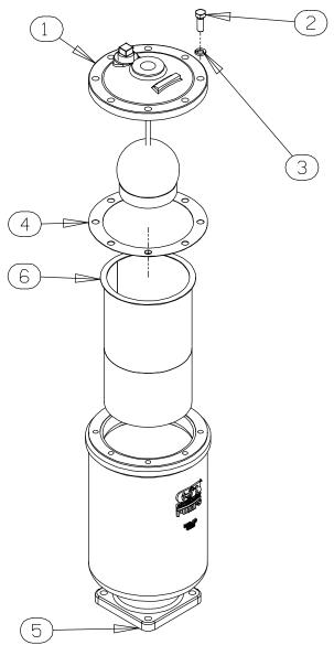
Figure 8. Priming Chamber Assembly
