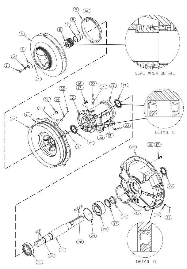
Figure 5. Repair Rotating Assembly
