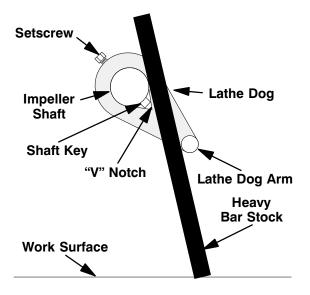
Figure 10. Blocking Shaft Rotation
