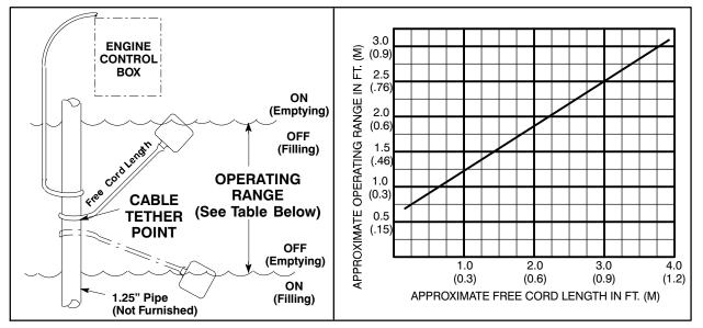
Figure 5. Float Switch Data
