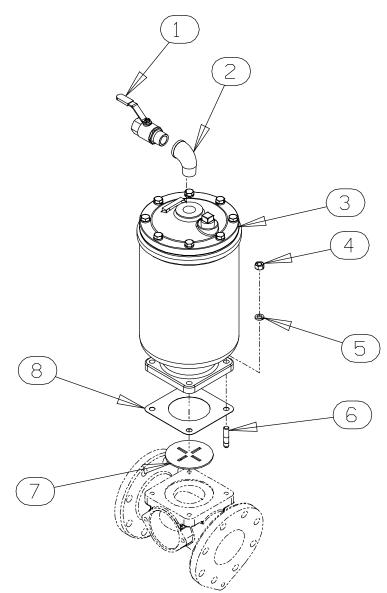
Figure 7. Priming Chamber Kit
