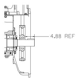
Figure 11. Drive Sprocket Positioning
