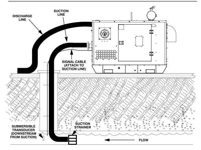
Figure 3. Typical Submersible Transducer Installation
