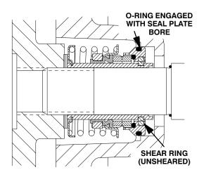
Figure 9. Seal Partially Installed
