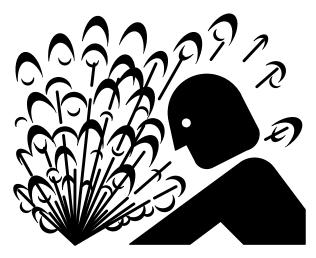
Natural Gas and Liquefied Petroleum Gas (LPG) presents an extreme explosion and fire hazard. Follow all safety precautions outlined by the National Fire Protection Association when designing and installing the system. Make certain that the regulators and fuel lines are of the proper size and capacity for the system, and that all fuel lines are securely connected and free of leaks.
