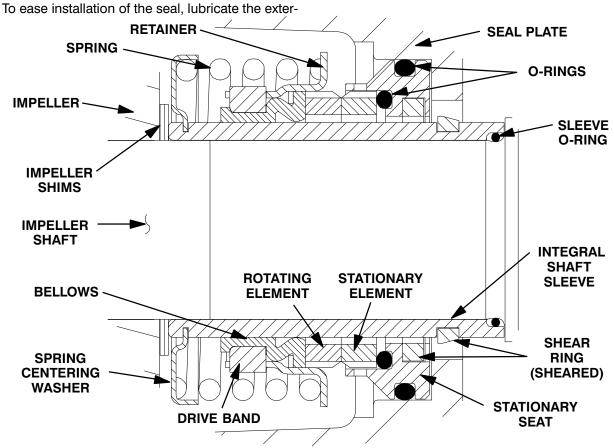
Figure 8. Seal Assembly
