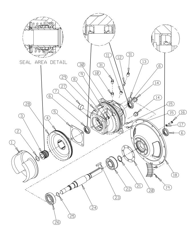
Figure 4. Repair Rotating Assembly
