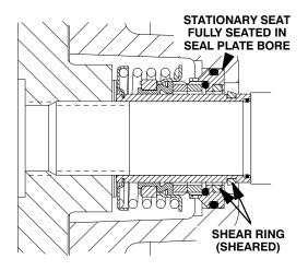
Figure 10. Seal Fully Installed
