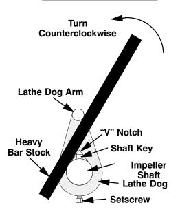
Figure 6. Loosening Impeller
