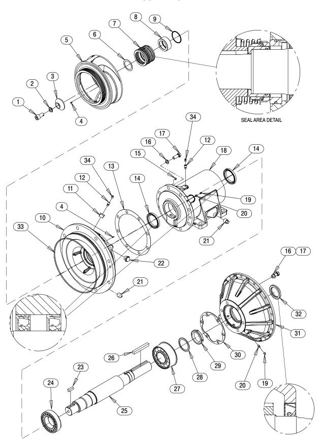
Figure 5. Repair Rotating Assembly
