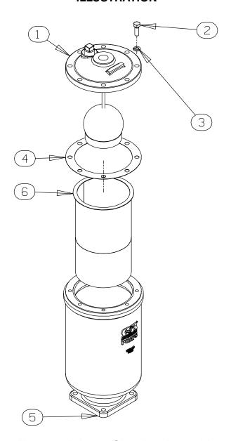
Figure 7. Priming Chamber Assembly PARTS LIST
