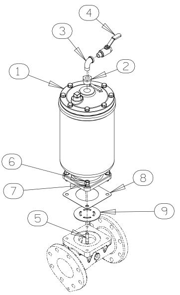
Figure 6. Priming Chamber Kit PARTS LIST
