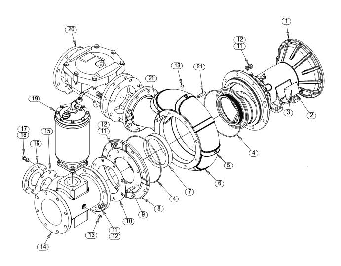
Figure 4. Pump End Assembly
