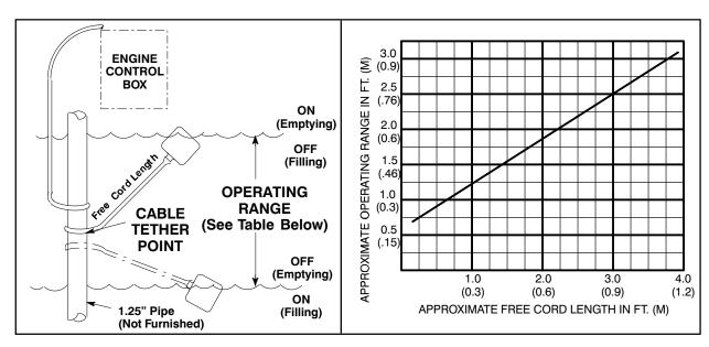
Figure 3. Float Switch Data
