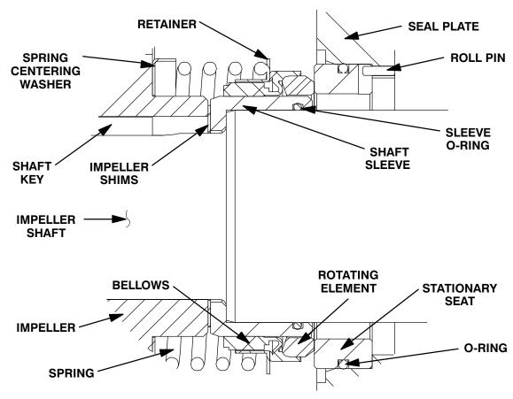
Figure 9. Seal Assembly
