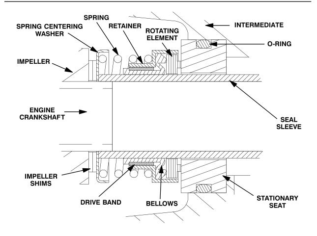
Figure 4. Seal Assembly
