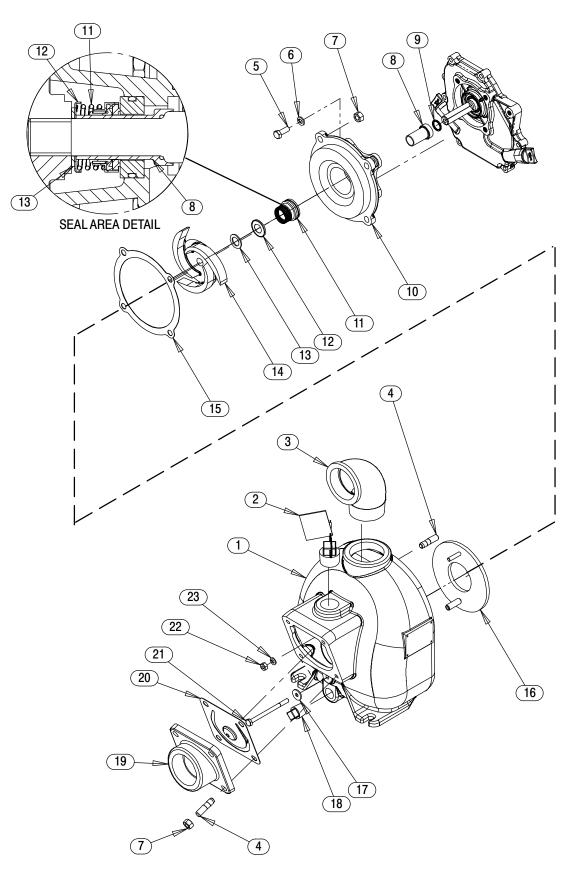
Figure 2. Pump Parts
