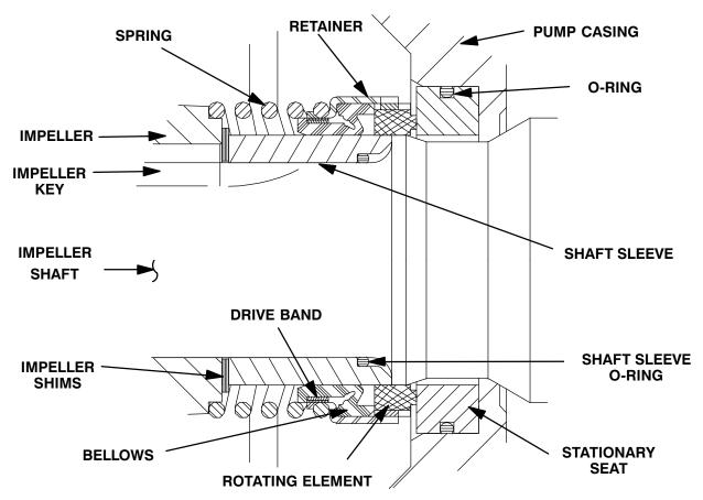
Figure 9. Seal Assembly
