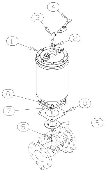
Figure 6. Priming Chamber Kit
