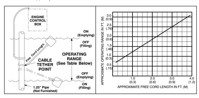
Figure 3. Float Switch Data
