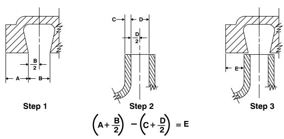
Figure 10. Centering Impeller Within Volute Scroll
