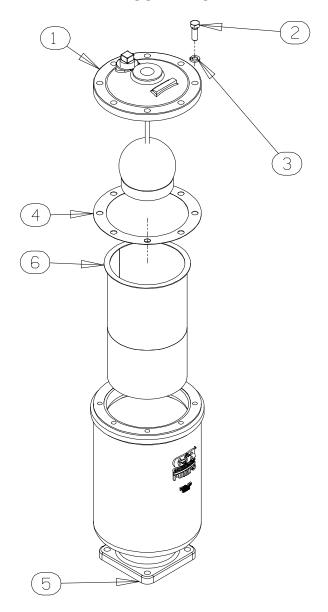
Figure 7. Priming Chamber Assembly PARTS LIST
