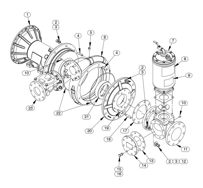
Figure 3. Pump End Assembly
