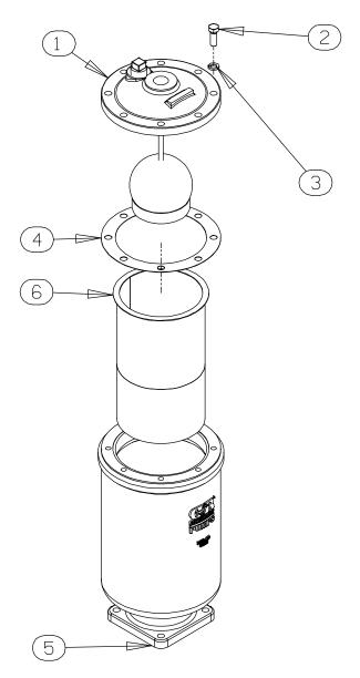
Figure 6. Priming Chamber Assembly PARTS LIST
