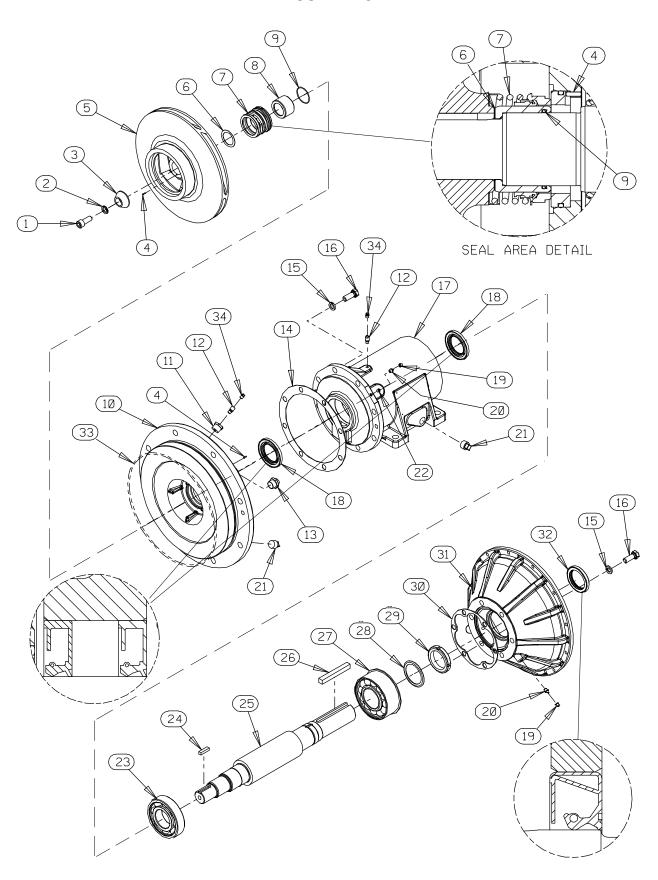
Figure 4. Repair Rotating Assembly
