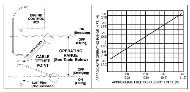
Figure 3. Float Switch Data
