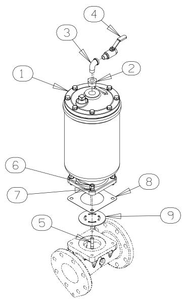
Figure 5. Priming Chamber Kit
