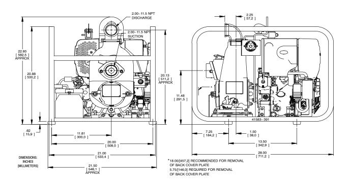
Figure 1. Pump Model 12D1-1B30E FT4 S/G
