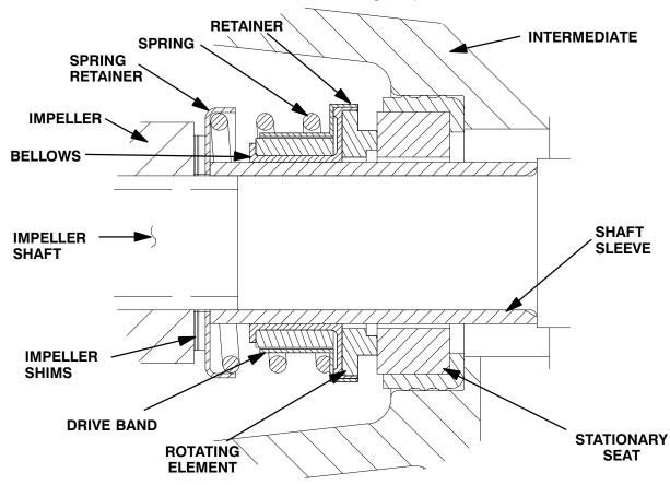
Figure 3. Seal Assembly
