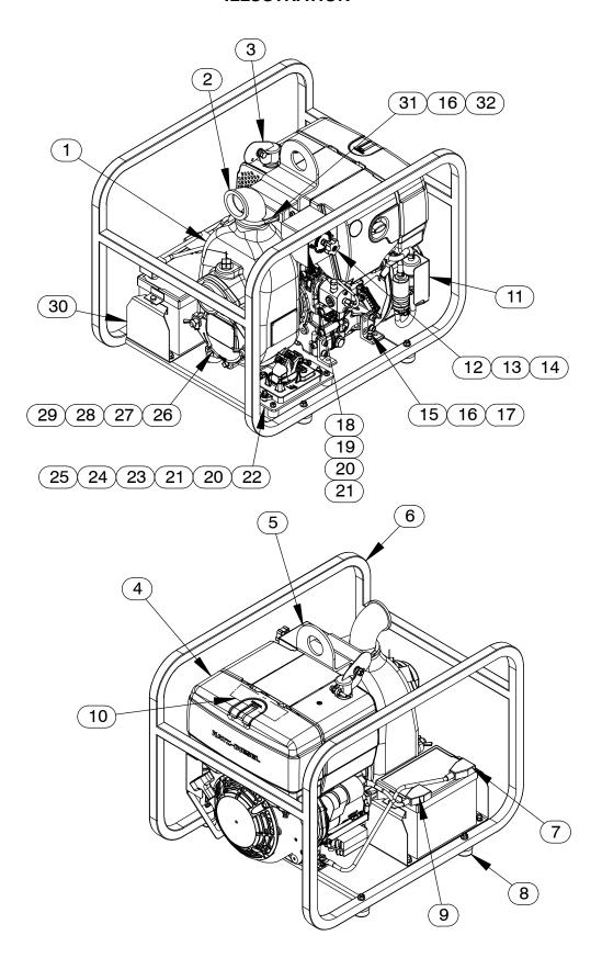
Figure 1. Pump Model 12D1-1B30E FT4 S/G
