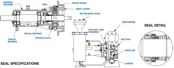
Seal: Mechanical; Self-Lubricated. Fluorocarbon Elastomers (DuPont Viton® or Equivalent). Carbon Rotating Face; Ni-Resist Stationary Face; Maximum Temperature of Liquid Pumped is 160°F (71°C).\*
