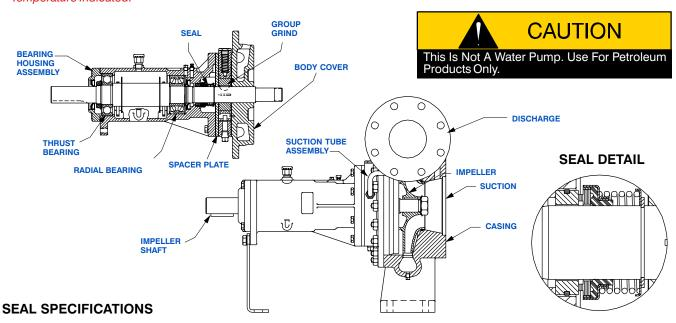
Seal: Mechanical; Self-Lubricated. Fluorocarbon Elastomers (DuPont Viton<sup>®</sup> or Equivalent). Carbon Rotating Face; Ni-Resist Stationary Face; Maximum Temperature of Liquid Pumped is 160°F (71°C).\*
