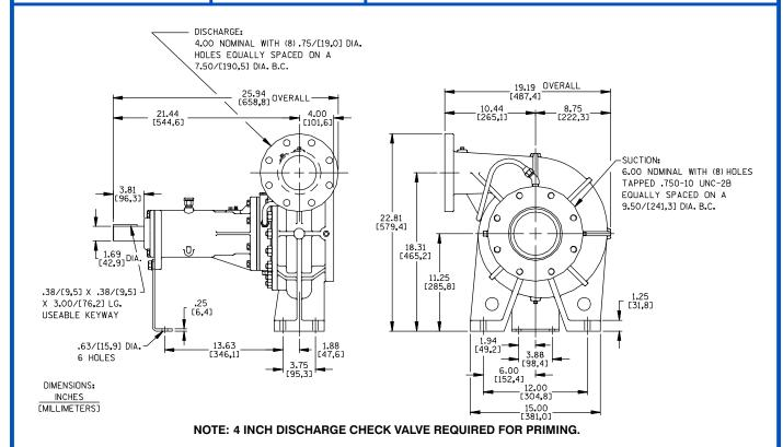
Air Release Valve Required When Static Discharge Pressure Exceeds 8 psi (55 kPa).
