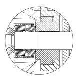
**SEAL DETAIL** Type 9, Mechanical, Self Lubricated. Tungsten Carbide Rotating and Stationary Faces. PTFE Elastomers. Stainless Steel 316 Cage and Spring. Maximum Temperature of Liquid Pumped, 160°F (71°C).\*
