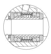
**SEAL DETAIL** Double, Grease Lubricated with Spring Loaded Grease Cup. Sintered Bronze Stationary Seal Seats. Steel Rotating Faces. Neoprene Packing Rings. Maximum Temperature of Liquid Pumped, 110°F (43°C). Maximum Suction Pressure 10 psi (69 kPa).\*
