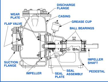
**SEAL DETAIL** Double, Grease Lubricated with Spring-Loaded Grease Cup. Sintered Bronze Stationary Seal Seats. Steel Rotating Faces. Neoprene Packing Rings. Maximum Temperature of Liquid Pumped, 110°F (43°C). Maximum Suction Pressure 10 psi (69 kPa).\*
