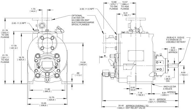
★ 18.00/[457,2] RECOMMENDED FOR REMOVAL OF BACK COVER PLATE T2CSC-B - 8.50/[215,9] REQUIRED FOR REMOVAL OF BACK COVER PLATE T2DS-B / T2ESC-B - 9.50 / [241,3] REQUIRED FOR REMOVOVAL OF BACK COVER PLATE
